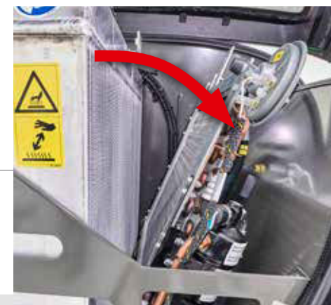
Very good accessibility to the radiator due to foldable condenser of the air conditioner / fuel cooler.
