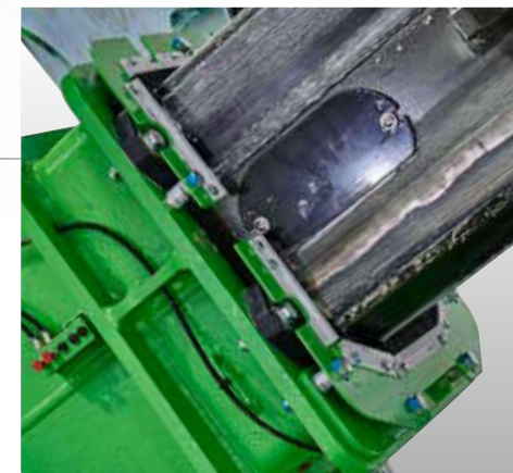
Telescopic boom slideways are accessible from the outside - easy maintenance and troubleshooting.
