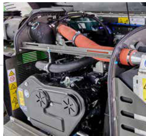
Easy access to all service points thanks to transversely mounted motor.
