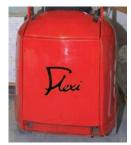
Detailed steel plate rear panel protects traction battery. Narrow 1000mm wide rear chassis allows block stacking and drive in rack operation.
