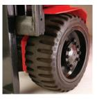
Flexi EURO front cushion rubber drive wheels provide excellent grip and traction in slippery conditions when fully loaded.
