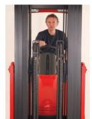
Operators have excellent forward visibility thanks to the triplex free lift mast, with its twin side mounted lift cylinders.
