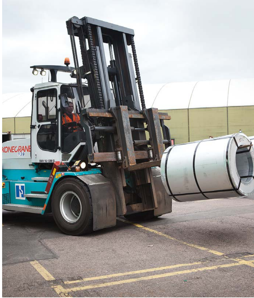
The SMV 4545 CBX5 reach stacker for intermodal handling can stack and lift 45 tons across all 3 rows.
