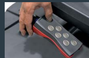
3 Pre-lowering load from the operating panel
