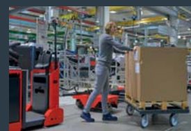
4 Unloading at destination, trolley taken to location, fill-up defined line-locations
