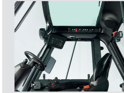
Armoured glass roof
